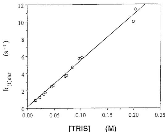
**Figure 2.** Plot of  $k_{\text{fast}}^{\text{obs}}$  vs  $[\text{TRIS}]$  for reaction of  $\text{Cr}_2\text{O}_7^{2-}$  at 25 °C and  $I = 1.0 \text{ M}$  ( $\text{NaClO}_4$ ).
