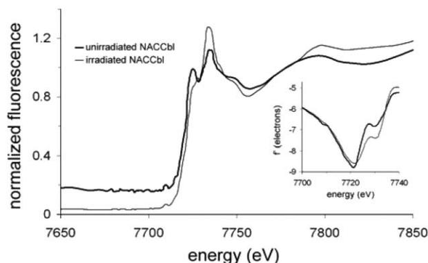
**Fig. 5** X-Ray absorption spectrum of unirradiated (bold) and irradiated Na[NACCbl]·18H<sub>2</sub>O between 7500 and 7900 eV. The inset shows the first derivative of the spectrum, with the negative peak position (7721.3 and 7721.4 eV for the irradiated and unirradiated samples respectively) corresponding to the position of the inflection point or threshold energy.
