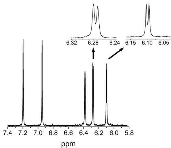
**Fig. 3**  $^1\text{H}$  NMR spectrum of D,L-homocysteinylcobalamin in  $\text{D}_2\text{O}$ , pD 5.9 (0.1 M MES buffer),  $22 \pm 1$  °C. Five major signals are observed at 7.20, 6.95, 6.38, 6.28, and 6.10 ppm, corresponding to the resonances of the B7, B2, B4, R1 and C10 protons (see Fig. 1).
