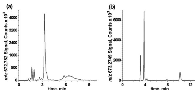
**Figure 10.** Plot of extracted ion signal in the  $m/z$  640–690 range versus time for the product solution formed from the reaction between HOcbl ( $8.0 \times 10^{-5}$  M) with 1.0 mol equiv  $\text{CO}_3^{\cdot-}$  at pH 9.00 (0.040 M  $\text{KH}_2\text{PO}_4$ , 0.080 M  $\text{KHCO}_3$ ,  $I = 0.20$  M, RT,  $\text{N}_2\text{O}$ -saturated buffer). Inset: Corresponding UV/Vis chromatogram of the product solution at 350 nm.
