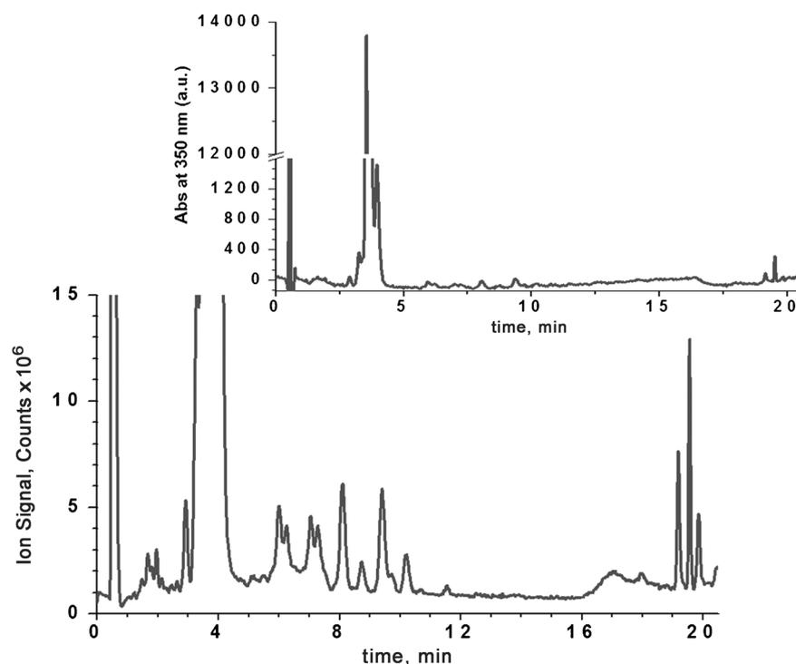
**Figure 11.** Plot of extracted ion signal for a)  $m/z = 672.783$  (corresponding to the doubly charged Cbl–2H complex, and b)  $m/z = 673.275$  (lactone derivative of  $\text{B}_{12}$ ) versus time for the products of the reaction of HOcbl ( $8.0 \times 10^{-5}$  M) with 1.0 mol equiv  $\text{CO}_3^{\cdot-}$  at pH 9.00 (0.040 M  $\text{KH}_2\text{PO}_4$ , 0.080 M  $\text{KHCO}_3$ ,  $I = 0.20$  M, RT,  $\text{N}_2\text{O}$ -saturated buffer).
